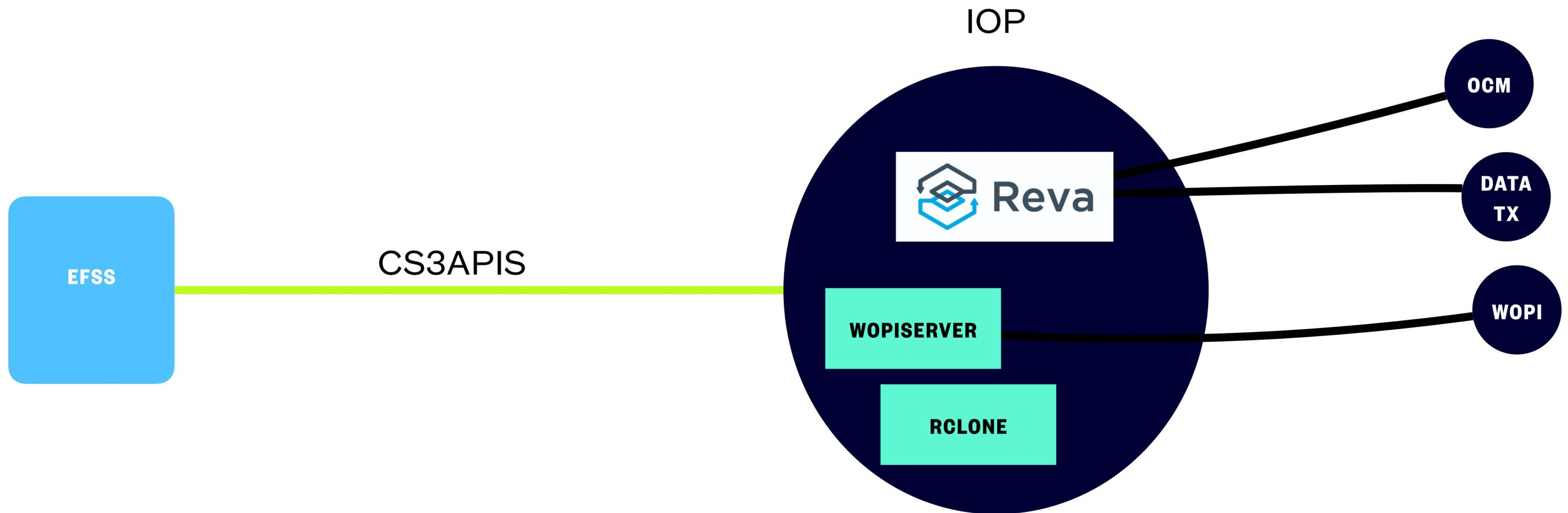
The IOP contains multiple components packaged into a K8S chart for easy deployment
