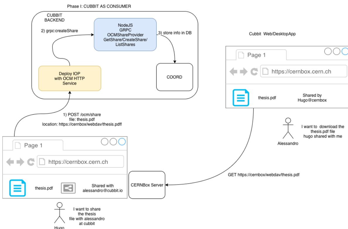
Figure 12. CUBBIT deployment with the IOP
