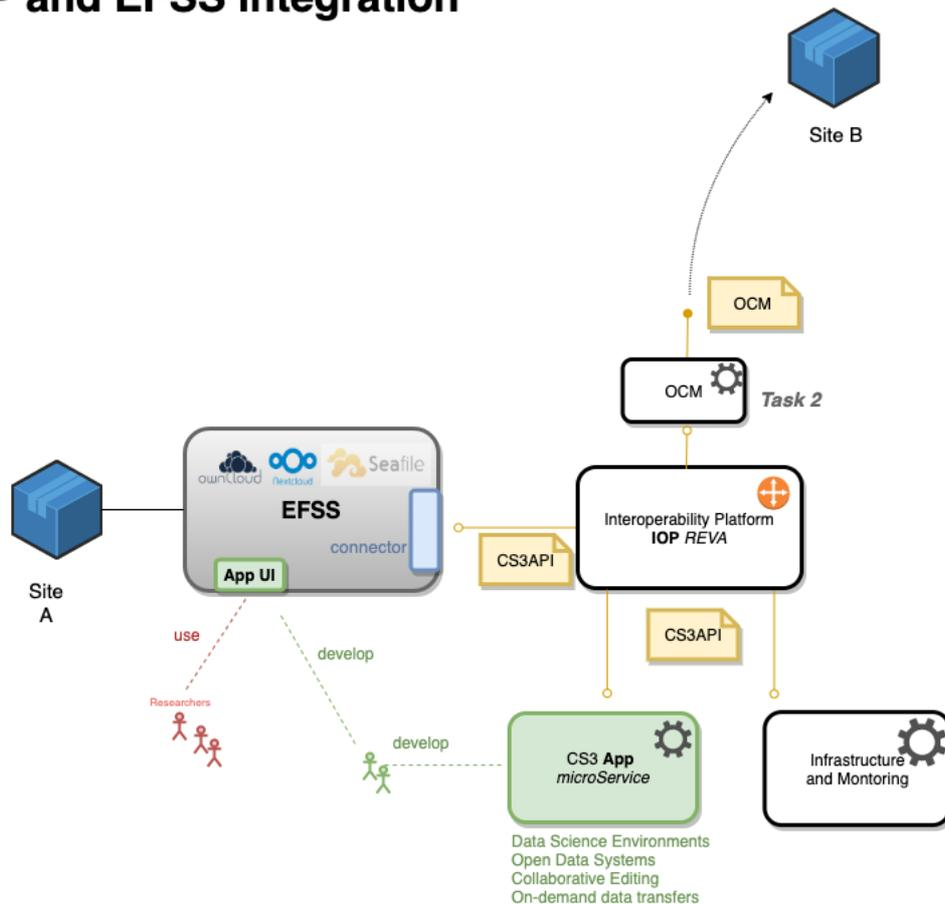
Figure 4. IOP and EFSS Integration Architecture
